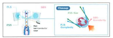
The hematology analyzer uses patented light scatter Technique to differentiate WBC population. When diluted blood is injected into flow cell. Blood cell passes through the sensing zone in a single file. A laser beam through the sensing zone is scattered by the passing cells and it is detected in three dimensional as follows.
