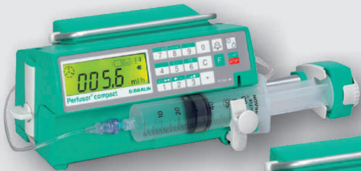
Perfusor® compact The user-friendly handy syringe pump for standard infusion therapy in all wards.
