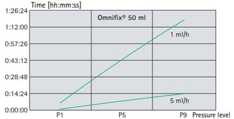
**Note:** At a rate of 0.01 ml/h the alarm time is > 4 h.
