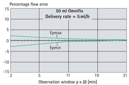
**Note:** Every syringe has certain tolerances in start-up behaviour (depending on the syringe manufacturer, syringe plunger material, siliconisation of the cylinder etc.).
