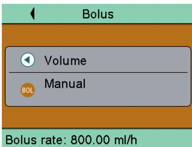
**Note:** If the bolus administration is not started after the Bolus key is pressed, the device automatically returns to the delivery screen for the ongoing infusion.
