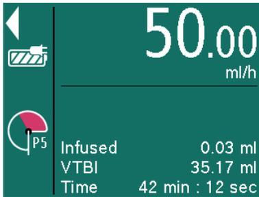
**Note:** The infusion rate set can be changed during an ongoing infusion by pressing the **OK** key.
